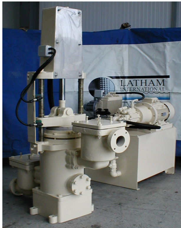
Refurbished Ram Pump
